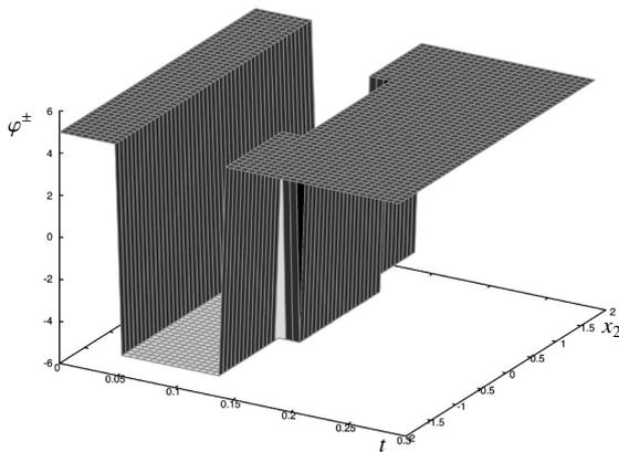
Fig. 6.1. The bang-bang feedback function  $\varphi_{\pm}$
