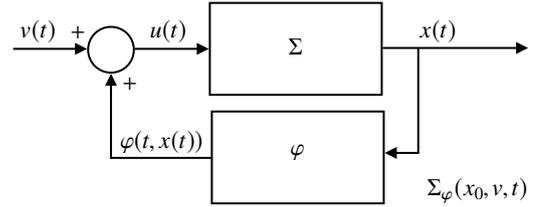
Fig. 3.1. Feedback system with external input
