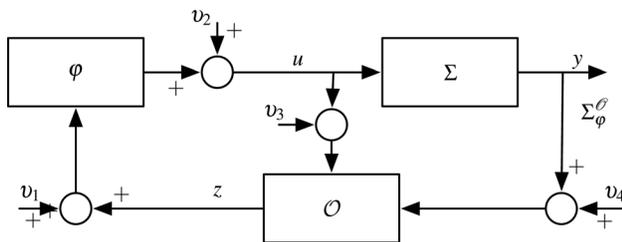
Fig. 6 Internal stability of the observer-controller configuration
