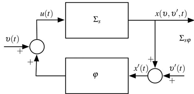
Fig. 7 Robust state feedback
