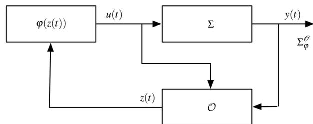
Fig. 4 The observer-controller configuration
