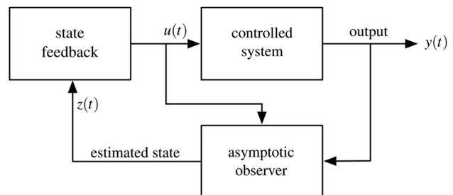
Fig. 1 The observer–controller configuration
