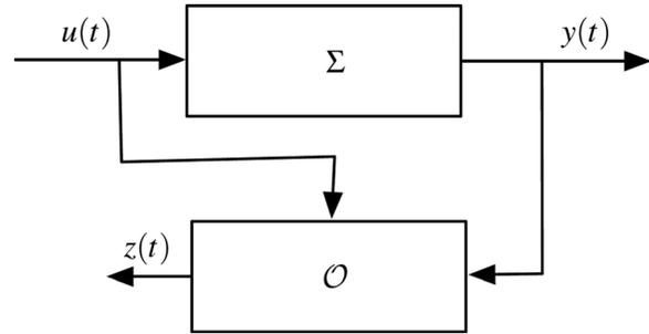
Fig. 3 An asymptotic observer  $\mathcal{O}$  for the observed system  $\Sigma$
